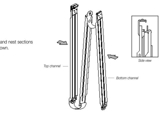
Fold channels and nest sections together as shown.
