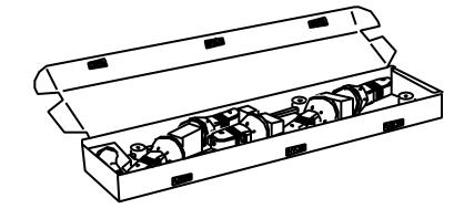
Attach SkyTrak fixtures to light cord (found in lid of Transporter case).
