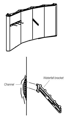
Waterfall Bracket Carefully pull panel away exposing channels. Insert bracket into channel notches and push down to lock into place.
