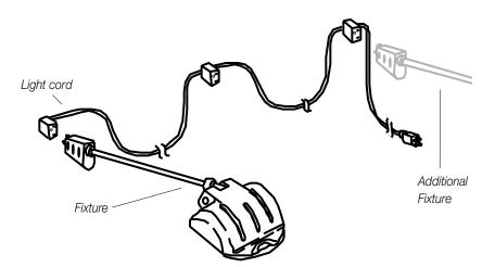
Attach fixture to clip on top section of channel. Hold down locking tab and back fixture into clip.
