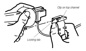
Rotate fixture 90° counter-clockwise.
