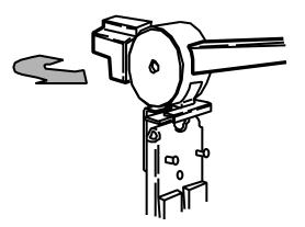
Place channels with light fixtures in desired position on frame (see right for typical placement).
