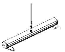
2. Connect pole sections and insert pole into hole in base.
